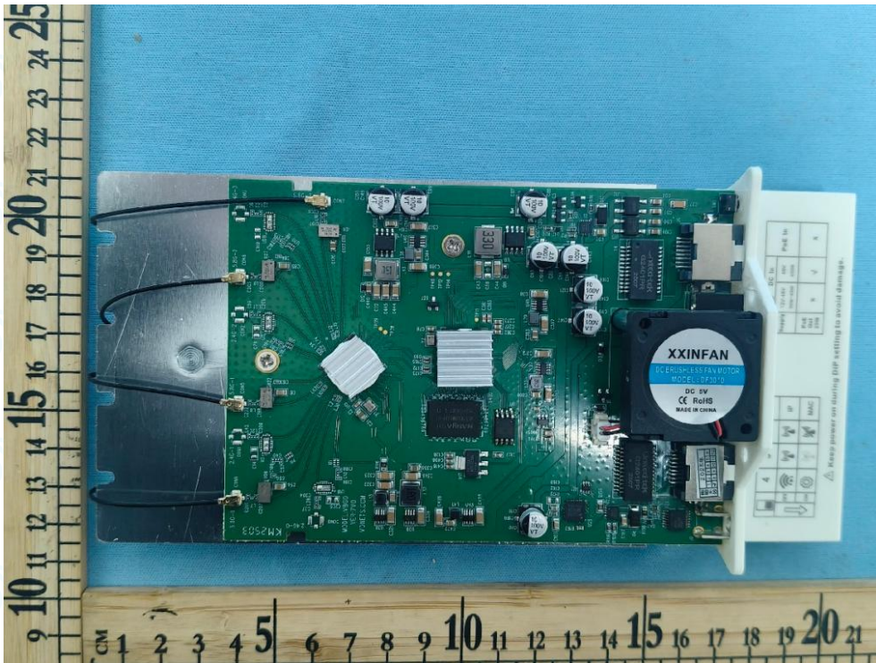
Figure 4: After IP6X test
