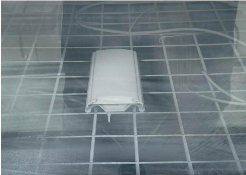
Figure 3: IP6X test on-going
